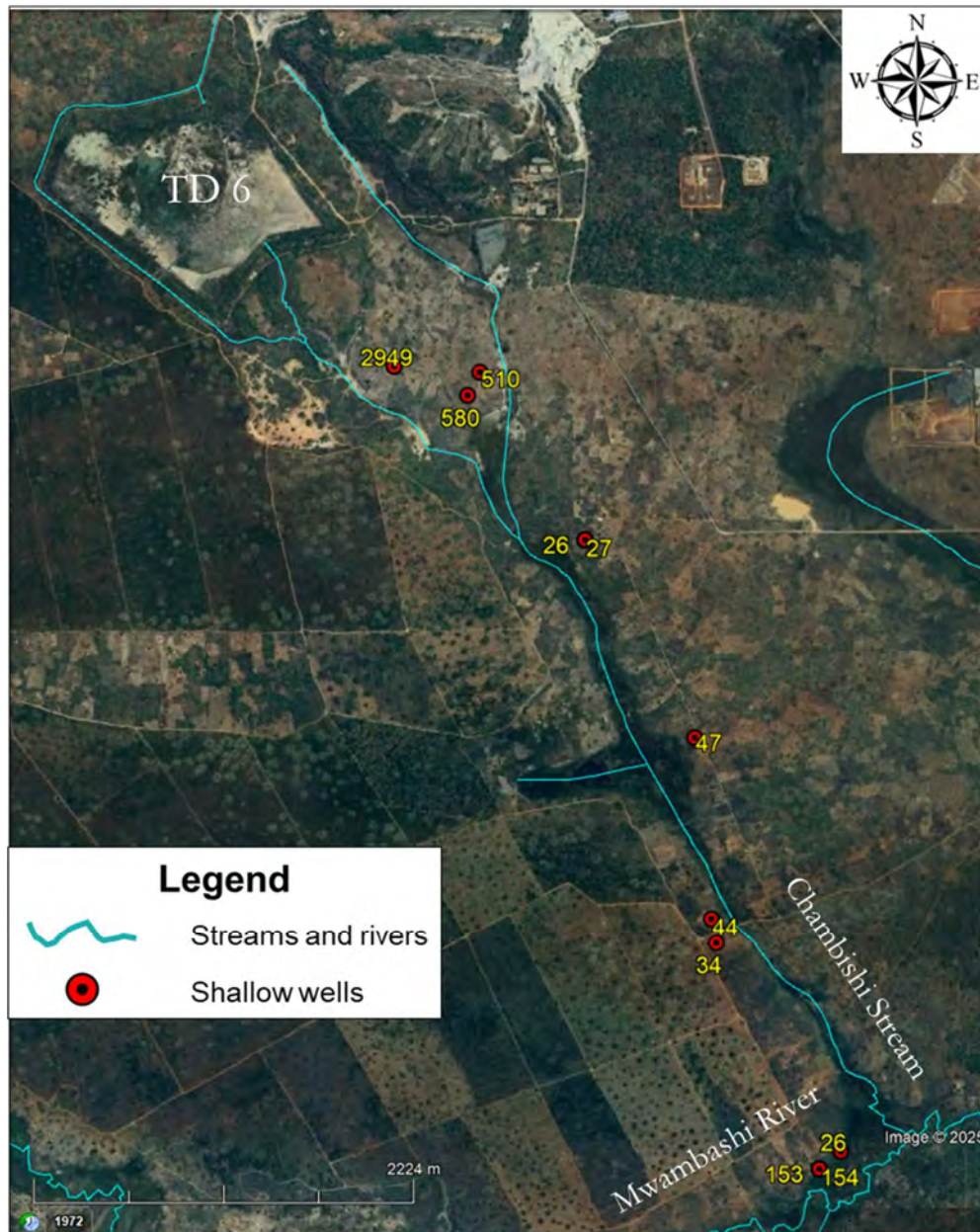
Figure 5-16: Satellite image showing the EC of shallow wells in the Kalusale area
