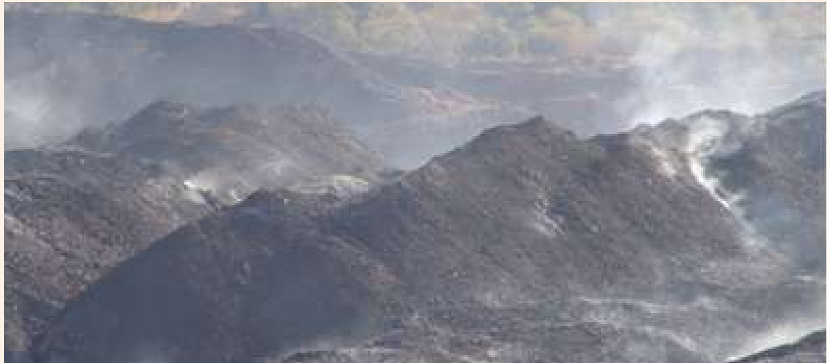
Overburden consisting mainly of carbonaceous and coaly mudstone showing spontaneous combustion affecting vegetation to the west, northwest and north in Izuma area, Maamba Mine area (Photo courtesy of Nyambe, 2007).
